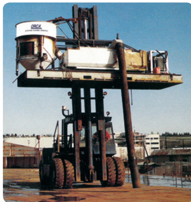
An example of using the Universal Hatch Cover™ to load sludge into the container from a Crowley barge.
